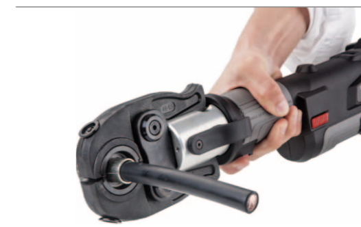
Crimping with 19KN from 16-300mm 2 for thin-wall terminals
