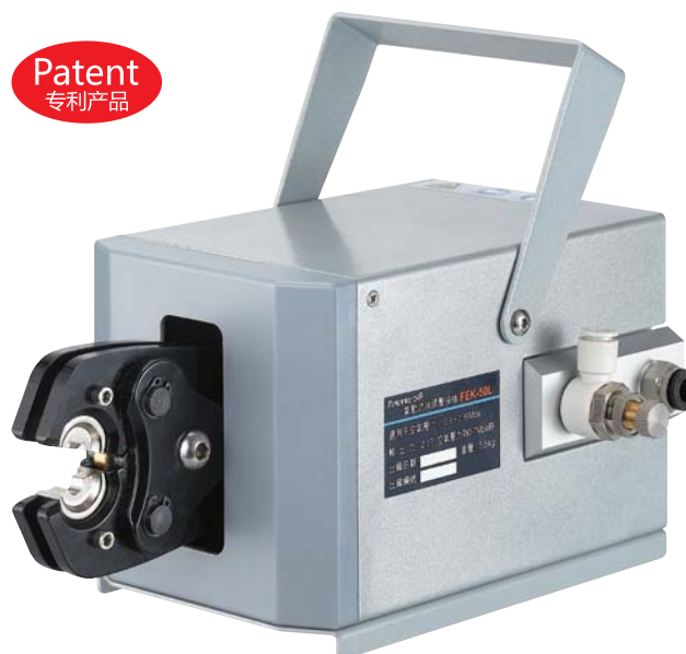
Terminal type: SC (Range: 6-95mm 2 ) TO (Range: 6-95mm 2 )
