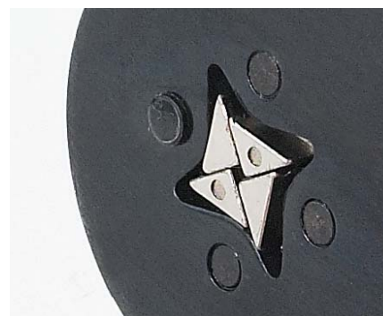
Self-adjusting adaptation to the desired end terminal (ferrule) size
