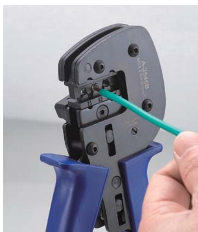
Then put the stripped insulated conductor into the terminal
