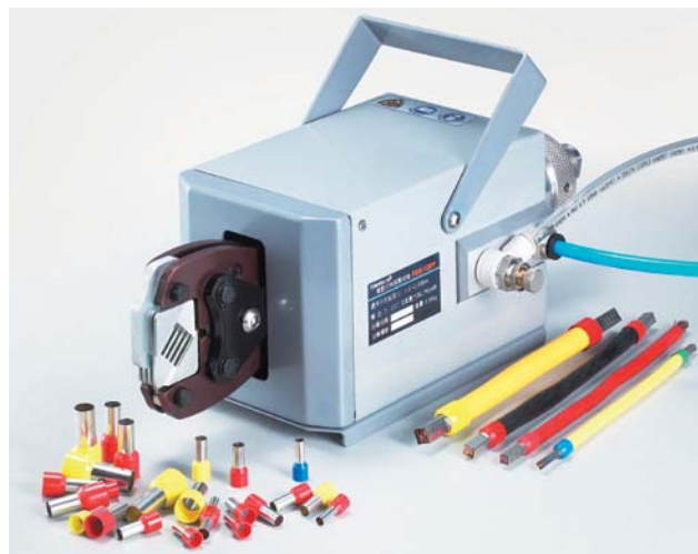
FEK-120Y Crimping die sets with front feed or side feed available for selection
