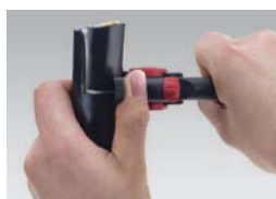
Rotate the tool and cutting around
