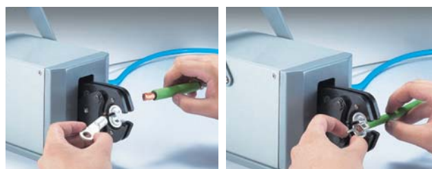
Terminal type: SC (Range: 6-95mm 2 ) TO (Range: 6-95mm 2 )
