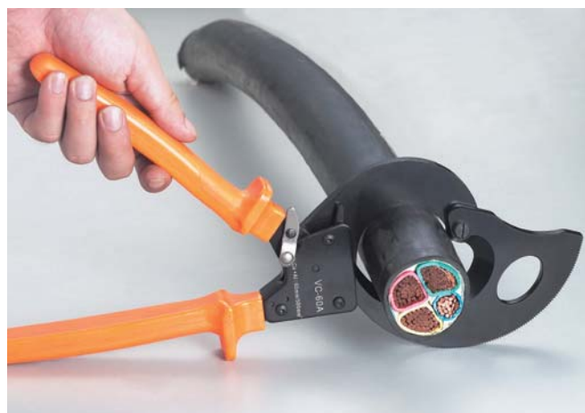
Cutting with one hand, fix the exit position of the handle on the plane surface and press down on the other handle
