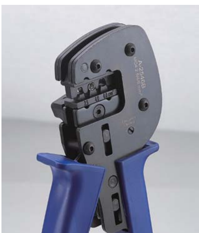
Put the terminal in relevant die set first
