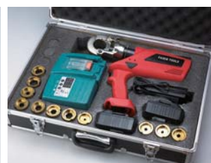
Change die set only after removing the battery
