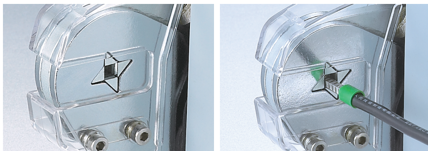
End, Twin End Terminals insertion at the side of the tool
