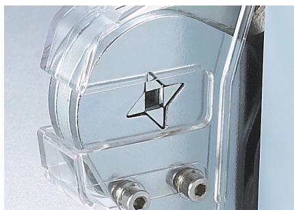
End, Twin End Terminals insertion at the side of the tool
